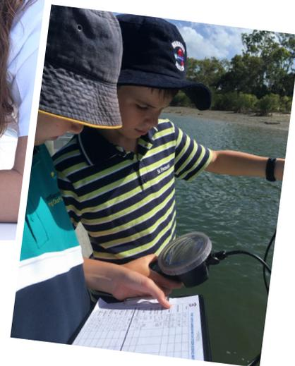
*To protect the multi-probe sensors, always use the guard and keep the probe off the bottom*
